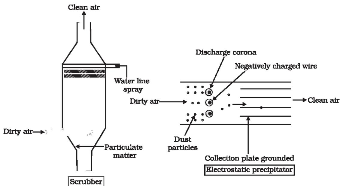
Figure 16.1 Electrostatic precipitator
